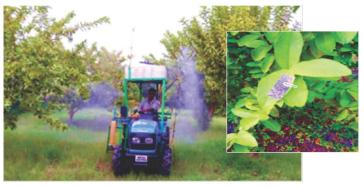
time of the spraying system were 475 l/ha and 12 s, respectively. The volume mean diameter (VMD) and volumetric spray deposition were 248  $\mu$ m and 0.291  $\mu$ l/cm², respectively.
