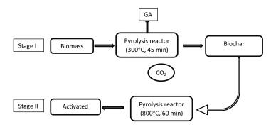
residues into activated charcoal. The crop residues generated from agricultural fields is a low cost material which can be used for production of activated carbon. Two step process and protocol to generate the activated charcoal from crop residues was developed at CIAE, Bhopal. The raw bio-material i.e. pigeon pea stalk was converted into valuable highly activated charcoal in two step process. In first step, the pigeon pea stalk was carbonized at 300
