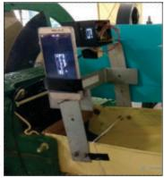
integrated. PIR Sensor has been fixed on the frame in such a way that it faces the feeding chute area. The data for human hand motion for different subjects at different distances and for different hand orientations has been collected by continuous video recording of OLED display.
