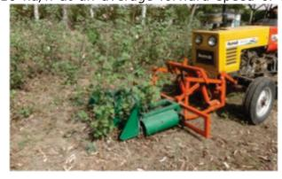
km/h with a field efficiency of 72 %. The machine can uproot 43-54 cotton plants per min. The stalk uprooting efficiency, percent stalk breakage ranged from 91.2 to 95.33% and 4 to 8%, respectively.
