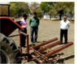
nism has been developed consisting of a screw type metering mechanism, power transmission system with chain and sprocket as well as ground wheel, stack for storage the seedlings and three point attachment system. The replaceable screw metering mechanism and stack have been fabricated so as to reduce number of seedlings fillings
