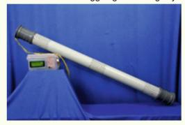
Sensor rod mounted with alert generation system
