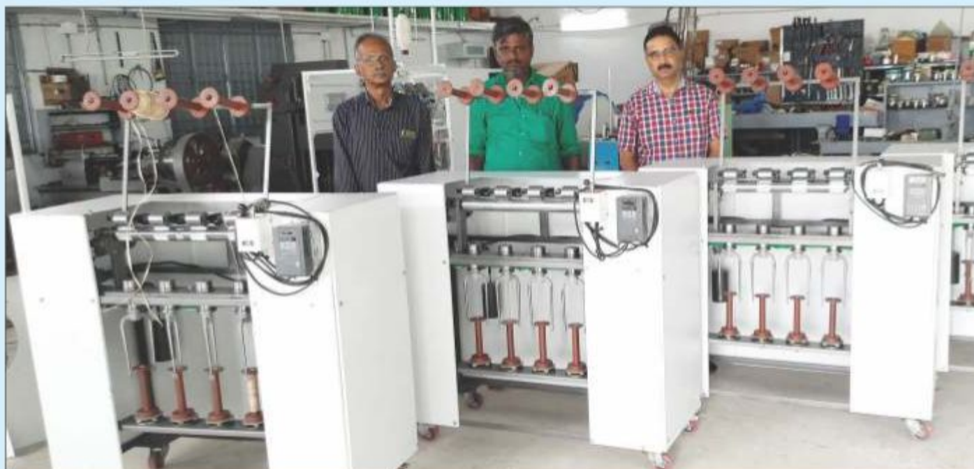
Commercial production of the banana outersheath twisting and winding equipment by manufacturer by licensing through Agri innovate, New Delhi
