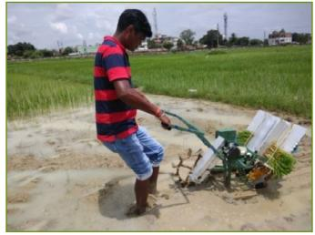
operated with less fatigue by an operator while the movement of the transplanting finger can be controlled with the help of switch provided on the handle.
