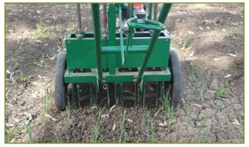
damage with the push type weeder are 91.21% and 6.81%, respectively. Push type onion weeder has been upgraded to self-propelled weeder by giving power from same 1.12 kw petrol engine to the wheels. Performance of weeder is found satisfactory during ongoing field trials. However, line transplanting of onion seedlings may be recommended for the best performance of weeder.
