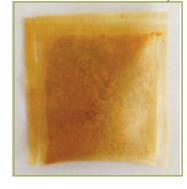
properties. The water barrier property of the film ranged from 5.3 to 9.2 x  $10^{-10}$  g/ ms Pa. The tensile strength of the film varied from 5.1 to 8.2 MPa, which is higher than similar composite edible films. The elongation of the film ranged from 70 to 88%. The edible film was
