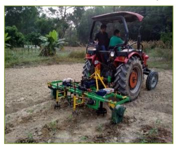
chili and tomato crops. The effective field capacity and field efficiency of sensor based inter and intra row weeder is 0.43 ha/h and 75% for wider row crop. The weeding efficiency of the machine is 90% in chili and 89% in tomato. The labour cost in weeding is reduced which ultimately reduces total cost of cultivation by 10-15%. Timely precise weeding in rows and between plants in chili crops increases yield and also saves soil nutrients consumed by unwanted weeds.
