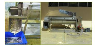
off material. The capacity of machine for *safed musli* peeling is 15-20 kg/h. The machine has potential to mechanize peeling operation of medicinal root crops and to reduce drudgery, labour cost and time.
