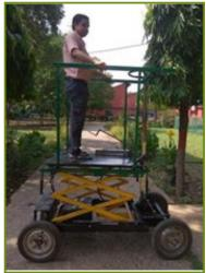
ratio of 1:9 in 10 s of time. However, the energy required to move 1.5 m is 600 Nm at forward speed of 0.54 km/h where lifting per stroke is 15 mm and total lift is 1200 mm. The energy required to lift the platform for change of stage (0.4 m) is 400 Nm. The use of developed platform enhances the reach of worker, reduces drudgery of pushing and pulling with ease of steering.
