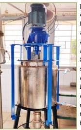
process. The pilot plant unit is capable of extracting dietary fibre from both soybean hull as well as chickpea hull with a capacity of 10 kg per batch and extraction efficiency of 80%. The biochemical analysis shows the total dietary fibre content of extracted dietary fibre from soybean hull and chickpea hull as 80% and 76%, respectively. The total cost for the establishment of dietary fibre extraction pilot plant is worked out as ₹2,96,400/- and
