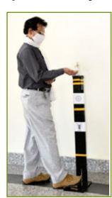
of sanitizer or liquid soap can be dispensed by pressing the foot pedal. Total height of the unit is 1100 mm. It is portable and can be placed at entrance of lobbies, corridors, farms, meeting rooms, outside the shops etc. The cost of this unit is about  $\gtrless$  1000/. This developed unit is being used for hand sanitization at different premises of the institute.
