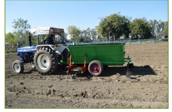
developed equipment is 0.44 ha/h with field efficiency of 80%. The functional testing of the machine has been completed; however rigorous testing in grape orchards will be carried out in next season.
