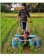
the developed system can be used for 5 different operations viz. wet land paddy weeding, row crop vegetable weeding, shallow tillage, digging small diameter pits and basin clearing for coconut tree. Paddy weeding attachment has also been developed for the multipurpose tool carrier which is powered by the 1.5 kW brush cutter engine.
