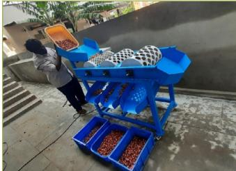
size of multiplier onion. The multiplier onion fed into the feed inlet passes to the rotating grading drums and the graded onion get collected at the respective outlets provided below the grading drums. The capacity of grader is 580 kg/h and is operated by 0.75 kW single phase electric motor.
