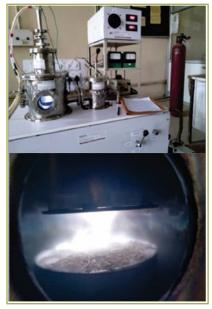
pirani gauge for vacuum pressure measurement, integrated three ways to control the vacuum inside the reactor. It can generate the vacuum as high as 10-8 bars. The thermal degradation behaviors of crop residues can be studied under different levels of vacuum and plasma intensity in different environment. Generation of free and charged radicals in plasma under different
