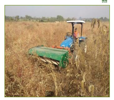
needed for efficient grass seed harvesting. It consists of the spiral bruising element on a rotary cylinder head which act as a grass seed collection mechanism. The machine has been tested in Dinanath Grass field at ICAR-IGFRI, Jhansi and its seed collection capacity found to be 5.5-6.0 kg/h, and the time required to fill the seed collection chamber is 40-45 min. The effective field capacity of the grass seed harvester is 0.1 ha/h at an average operating speed of 3.24 km/h for Dinanath grass.
