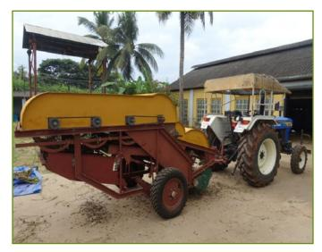
threshing system. The threshing and conveying efficiency of the picker combine is found to be 99% whereas the maximum stripping efficiency is 95% at 4 days after harvesting. It has been observed that, the entire plant mass is picked up by the header and conveyed into the threshing cylinder without any damage to kernals and pods.
