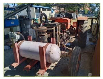
distributor and fitted/aligned in the timing gear mechanism of the tractor with modified flange. An inlet air manifold has been fabricated and carburettor has been suitably fitted to regulate the air-CNG mixture. All the arrangements with air cleaner have been made to connect carburettor and air cleaner. Further arrangements are in progress to operate the tractor engine with 100% CNG.
