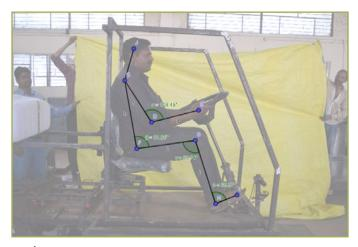
mm) and the range of trunk, elbow, hip, knee and ankle angle and overall dimension of workstation has been made to suit most of the drivers. All the prime mover controls viz. steering, brake, accelerator, etc. are suitably placed within operator reach envelope.
