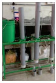
thus been kept as 15-25 mm for gravel, 5-8 mm for grit and 0.3-0.8 mm for sand. The filter media column made of PVC pipe of 110 mm diameter and 1.2 m height (1 m test height) has been used. The wastewater is pumped using peristaltic pump at lower end of the column, passed through vertical column and discharge is collected at the top end of the column. Experiments
