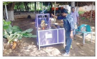
roots before placing it on the holder for trimming. The equipment is best suited for large size suckers. The capacity of the equipment is about 120-150 suckers per hour, the overall size of the equipment is  $1145 \times 515 \times 1825$  mm. The cost of the equipment is Rs. 80,000/-.
