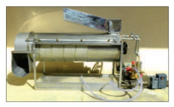
drive, as per the requirements of individual crop. The machine can peel 5 kg of freshly harvested *Shatavari* or *Safed musli* tuber roots in 10-20 min, thus significantly reduces the peeling time as compared to manual peeling. It also eliminates requirement of any kind of pre-treatments. The peeling efficiency has been observed as more than 90%, with minimum breakage to the crops. The machine can significantly reduce drudgery, labour cost and time.
