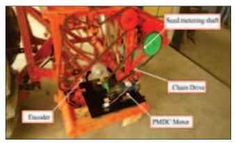
developed seed sensing system is capable of detecting the metered seeds.
