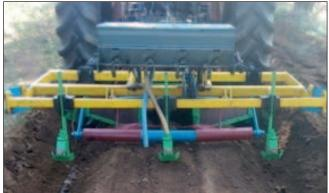
the weeding and other operations can be done easily without disturbing the bed configuration. About 15-35% increase in yield has been reported with the use of this equipment in black and sandy loam soils across different villages. It reduces the energy requirement by 35% compared to the conventional seed drill followed by weeding operations.
