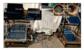
the various samples prepared, the best stable  $Al_2O_3$  nano-fluid is found for the combination of  $Al_2O_3$  (0.02%) + surfactant (0.01%) with four hour sonication. In case of Fe<sub>2</sub>O<sub>3</sub> nano-fluid, the stability period has been significantly short. The efficiency of the collector with nano-fluids is found over 40%, while the efficiency of the collector without nano-fluid remains 5% lower than the nano-fluid based collector.
