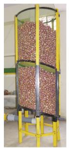
days in control storage. At the same time losses are 26.66% weight loss, 14.20% rotting and 5.88 % sprouting reported by other studies after 120 days storage. The structure is rust proof and hence expected to have long life and durability due to FRP material as major construction material. The time required for filling up and emptying the storage cage is about 0.83 man-h/t and 0.4 man-h/t, respectively as compared to 1 man-h/t and 3 man-h/t in case of conventional Chawl structures.
