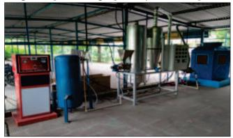
bio-oil by MPUAT, Udaipur centre. The system comprises of fluidized bed reactor, cyclone separator, condenser and cooling tower. Performance of developed system has been carried out with wheat straw, maize straw, and sugarcane bagasse as feedstock. The maximum bio-oil was obtained with biomass particle size of 1 mm at 450-500 °C.
