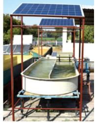
60 V and 6.9 A, respectively. Time required for harvesting is 4 h to bring down optical density of microalgae from 0.98 to 0.16 and harvesting efficiency varies from 81 to 86% during the different harvestings throughout the year. Averege energy consumption for electro-flocculation is found to be 3 kWh/kg of dry microalgae biomass.
