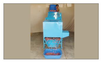
provided at the side for removal of the dust, dried and dead skin of onion. The maximum cleaning efficiency of 98% is obtained at 10.41m<sup>3</sup>/s air flow. The capacity of the cleaner is found to be 800 kg/h.
