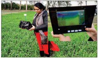
on screen. The maximum, minimum and mean temperatures in winter wheat crop at CRI stage are found to be 22, 14 and 14.75 °C, respectively. The temperature resolution is 0.25 °C and measurement accuracy is 2.5 °C. The developed imager can be utilized for crop stress monitoring and real time application of irrigation scheduling.
