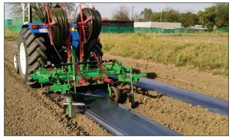
The drip lateral-cum-plastic mulch layer is suitable for variable width of raised bed, plastic mulch (1000-1500 mm), various drip lateral diameter different width of (<30 mm), soil properties, etc. It has been found that the field capacity and field efficiency of developed machine are 0.26 ha/h and 65%, respectively.
