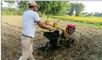
attachment to a walk-behind type of power tiller. Adjustment has been provided in furrow opener to operate at different depth. An average seed spacing of the planter has been observed as 250 mm, depth of operation as 25-45 mm and actual field capacity of 0.074 ha/h.
