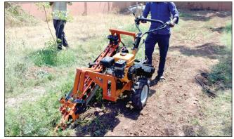
field capacity and field efficiency are 0.028 ha/h and 78.7%, respectively.
