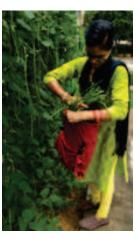
working height of 440 mm, unloading height of 700 mm, width of 200 mm and shoulder strap length of 1300 mm.
