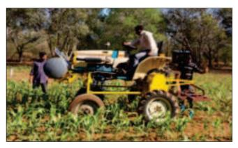
tasted in castor, pigeon pea and maize crops. The weeding efficiency of rotary weeder is found to be 82.5%. The approximate cost of the machine is Rs. 30,000/- and its operating cost is Rs. 600 /h.
