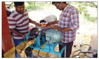
Cashew Apple Slicer - Vertical feed and horizontal slicing blade model
