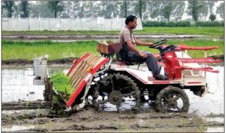
the time of transplanting. The performance parameters of rice transplanter with deep placement fertilizer applicator such as fertilizer application efficiency, field capacity and field efficiency are found to be 71%, 0.16 ha/h and 82%, respectively.
